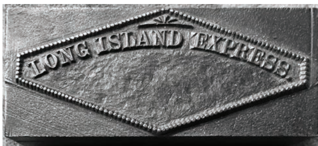
Figure 63. Relief-printing die. Mirror image of the printing surface is shown.
